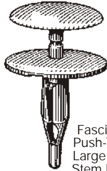
18269 (6503106) Black Nylon Lower Sill Moulding Push-Type Retainer Large Head Dia.: 7/8" Stem Length: 1" Fits Into 1/4" Hole Jeep Grand Cherokee Laredo 1994-On UNIT PACKAGE: 15
