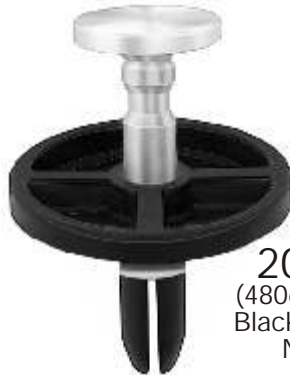
20940 (55157330-AC) Black Nylon Tail Light Push-Type Retainer Large Head Diameter: 31mm Small Head Diameter: 20mm Stem Length: 21mm Fits Into 8mm Square Hole Jeep Commander 2006 - On UNIT PACKAGE: 15
