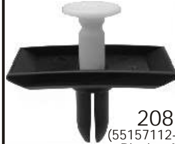
19638 (Chrys: 4805405AA; Ford: 1L5Z-17K826AA) Black & White Nylon Front Bumper Fascia Push-Type Retainer Head Dia.: 34mm Stem Length: 20mm Fits Into 8mm Hole Concorde, Intrepid, Eagle Pacifica & PT Cruiser 1998-On Ford Trucks 2005-On UNIT PACKAGE: 15
