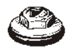
16134 Zinc & Yellow Thread Cutting Nut With Sealer For 3mm Stud 13.5mm O.D. 8mm Hex UNIT PACKAGE: 25
