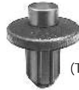
19219 (90467-09096) Black Nylon Front Bumper Push-Type Retainer Head Diameter: 15mm Stem Length: 27mm Fits Into 9mm Hole Lexus LS400 1993-On Celica & Supra 1989-On
