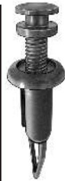
19219 (90467-09096) Black Nylon Front Bumper Push-Type Retainer Head Diameter: 15mm Stem Length: 27mm Fits Into 9mm Hole Lexus LS400 1993-On Celica & Supra 1989-On
