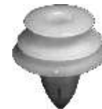
20575 (67771-12080) Yellow & White Nylon Door Panel & Rocker Moulding Retainer Top Head Diameter: 13mm Middle Head Diameter: 16mm Bottom Head Diameter: 18mm Stem Diameter: 10mm Stem Length: 13mm Overall Length: 20mm Toyota & Lexus 1998 - On
